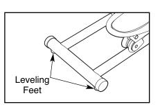
beneath the front stabilizer until the rocking motion is eliminated.
